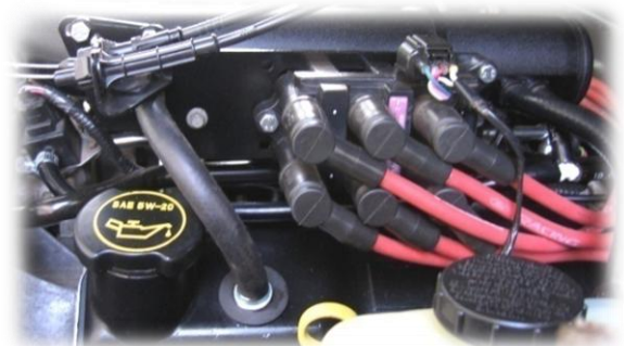
Side bracket with coil pack installed
